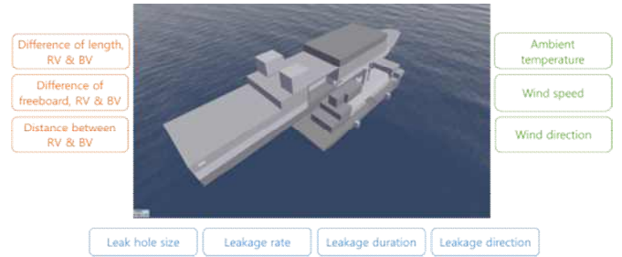
Fig. 5 Key parameters of leakage and dispersion analysis
