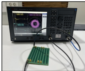
Fig. 4. S11, S21 Measurement using Network Analyzer.
