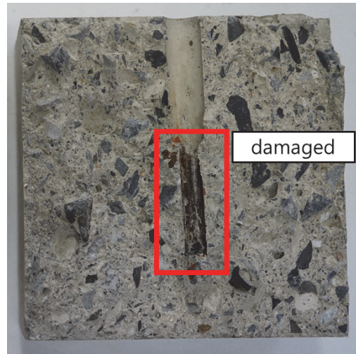
Fig. 8 Bond-slip destruction pattern: Type 1
