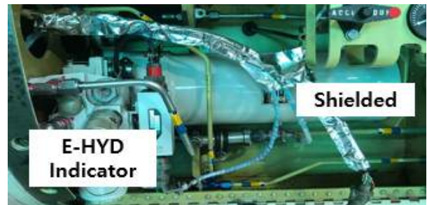
Fig. 17 Shielded W/H Path of the E-HYD Indicator
