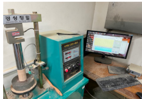
Fig. 3. Sample curing and uniaxial compressive test apparatus
