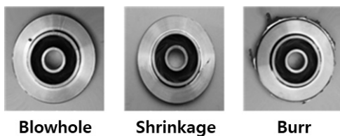
<Figure 4> 3 Defect type of Impellar
