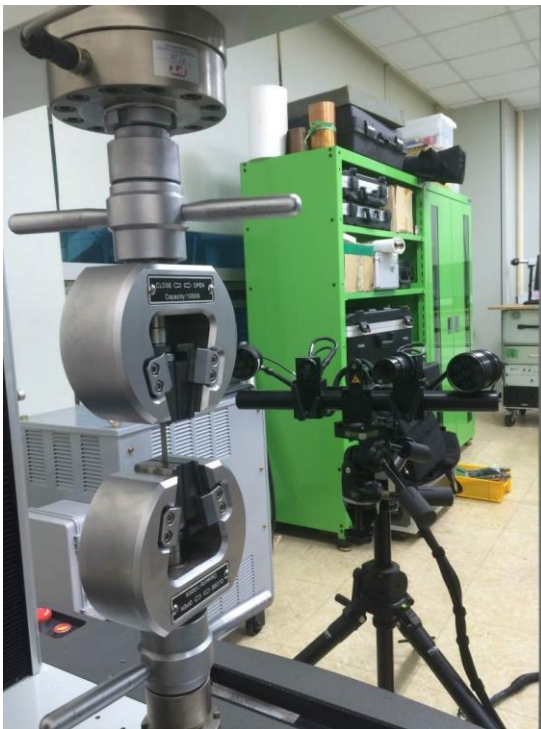
Fig. 1 Experimental set-up using the universal testing machine with ARAMIS 3D DIC system
