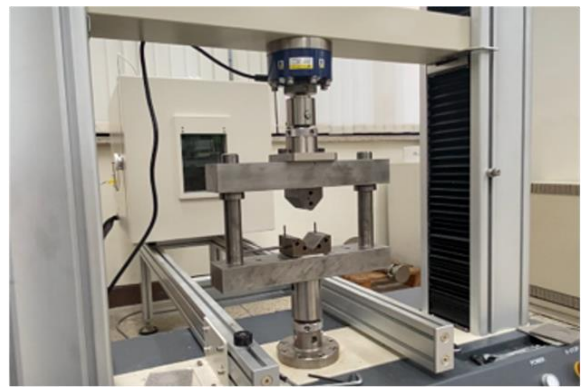
Fig. 7 Experimental set-up for the V-bending
