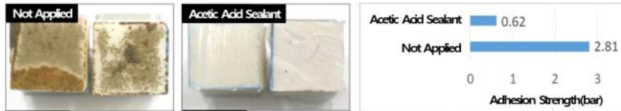
Figure 11. Surface and Adhesion with and without Application of Release Agent
