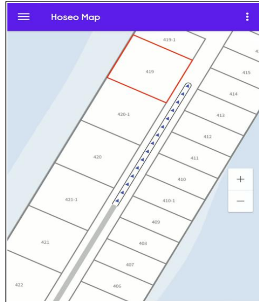
Fig. 6. Tracking of the user's indoor location and display of the route traveled
