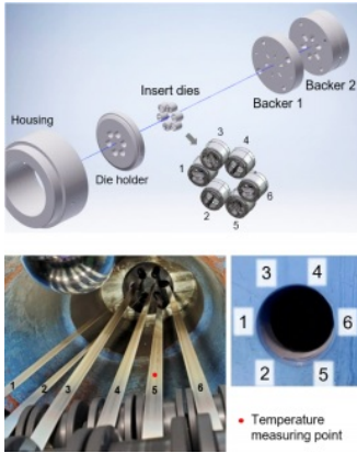
Fig. 2 Multi-port extrusion of micro-channel flat tube
