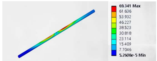
Fig. 8-1. Pipe stress at S1
