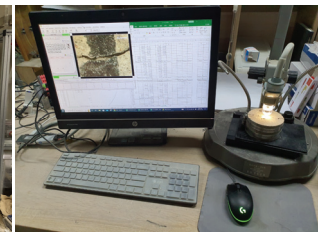
Fig. 6. Crack surface observation test
