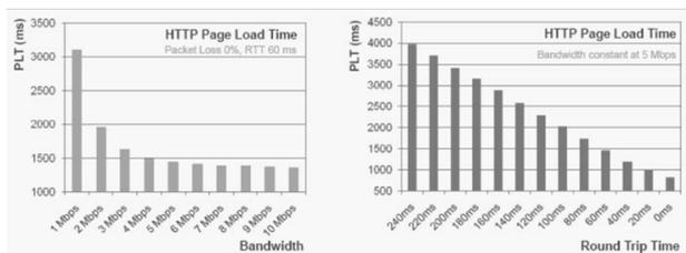
Fig. 5. Changes of Page Load Time by bandwidth and round trip time changes[4].
