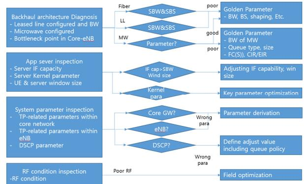
Fig. 10. Backhaul Network Diagnostic Procedure.
