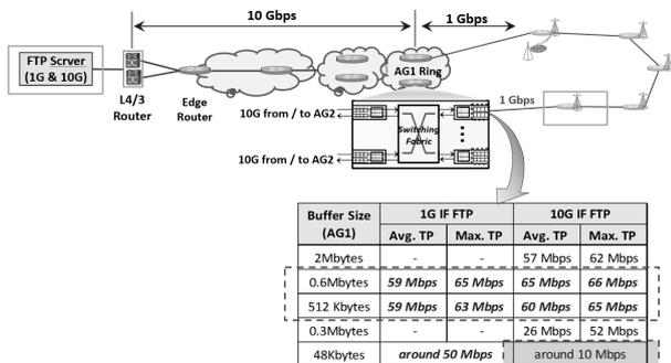
Fig. 8. Bottleneck diagnosis between eNB and AG through buffer size adjustment.
