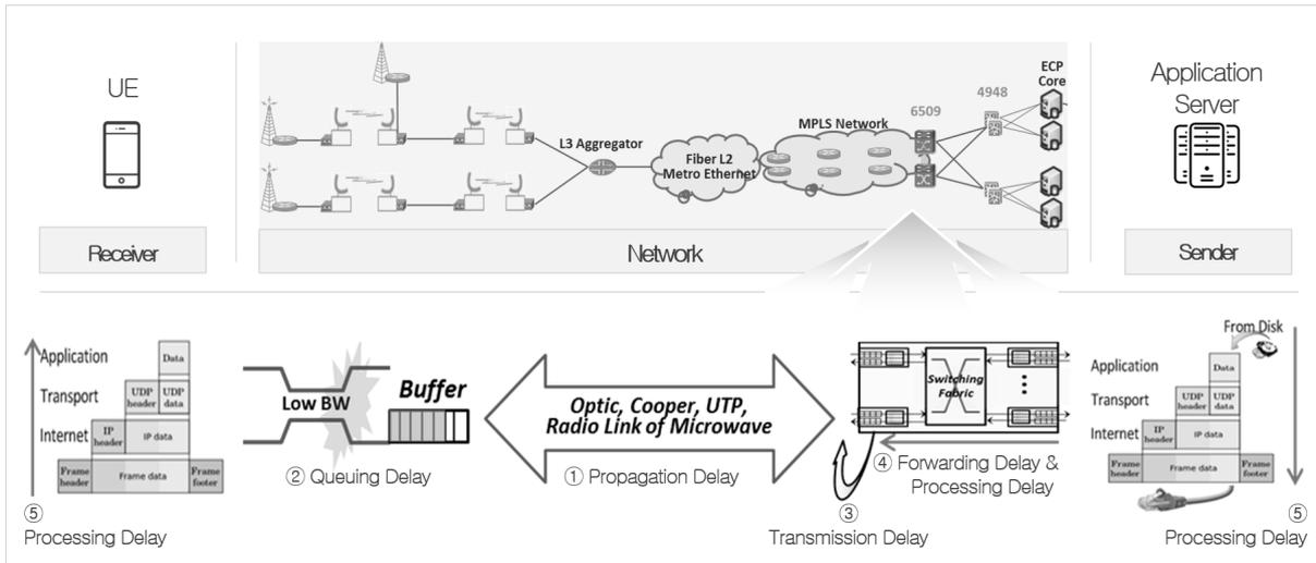
Fig. 6. End to end delay time.
