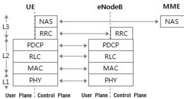
Fig. 3. LTE user plain and control plane protocol stack.
