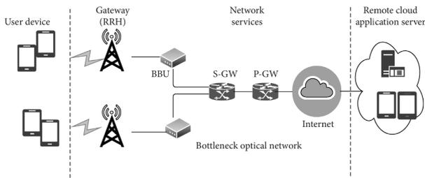
Fig. 1. Mobile communication architecture.
