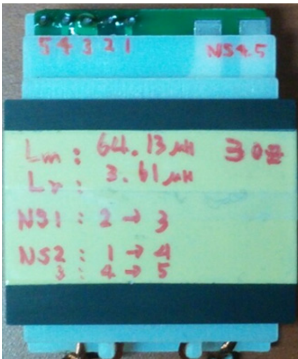
Fig. 15. Actual sample of high frequency LLC transformer with 3oz PCB and copper plate windings.
