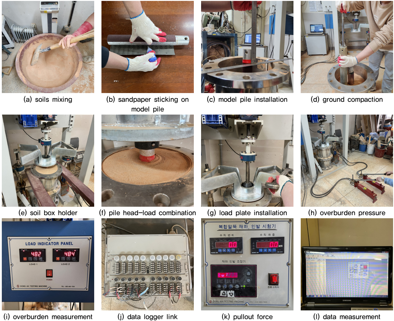
Fig. 4. Pullout test procedure and measurement
