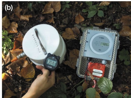
Fig. 2. Schematic diagram of the collar and cap for soil respiration measurement (a), and measurement of soil respiration and environmental factors (b).
