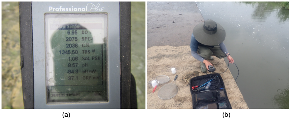
Fig. 2. Water quality measurement device (a) Multi Sensor Meter, (b) Water quality survey.
