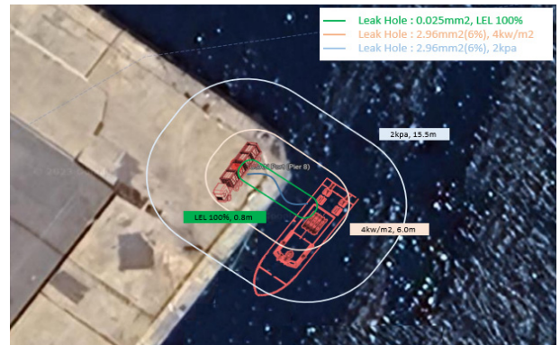
Fig. 7 Effective distance in case of 0.025mm 2 and 6% rupture of hose cross sectional area
