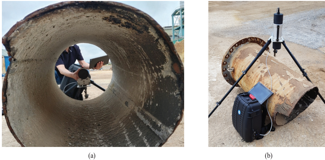
Fig. 4. In situ measurement of the scrap pipe with the MARK-B2 detector at (a) the central position and (b) the outside of the pipe.
