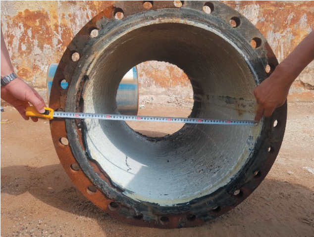
Fig. 1. The scales in the discharged scrap iron pipes during maintenance period of the \text{TiO}_2 processing factory.
