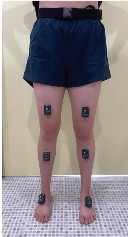
Fig. 1. Attachment of inertial measurement unit for assessment of lower extremity kinematics..
