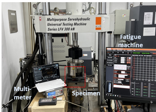
Fig. 2 Overview of piezoresistive test setup
