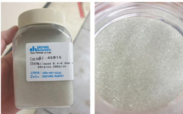
Fig. 5. Glass bead used to analyze the accuracy of PTV settling velocity measurements (diameter : 0.4~0.6 mm,  $\rho = 2.5$  g/cm<sup>3</sup>).
