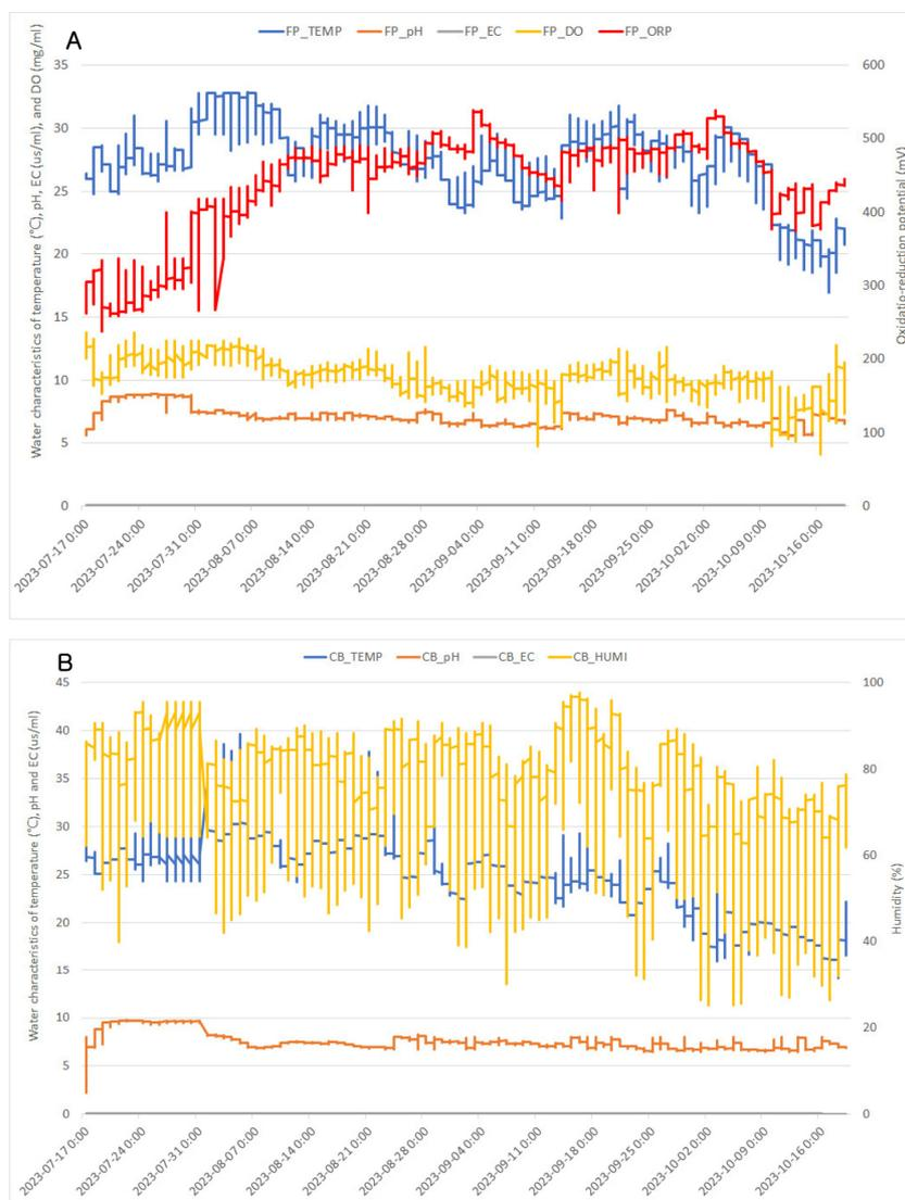
Fig. 2. Monitoring of water characteristics, temperature, pH, EC, dissolved oxygen (DO), and oxidative-reduction potential (ORP) of cattfish culture pond (A) and crop culture bed (B) for aquaponics systems for lettuce and chicory.
