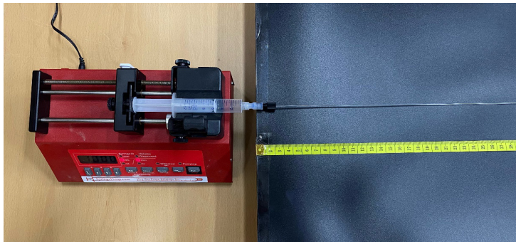
Fig. 8. Experimental setup of grouting injection
