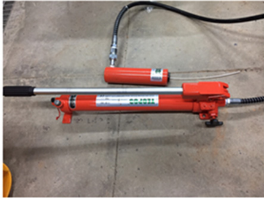
Fig. 5. Measuring instrument for rock bolt pullout capacity
