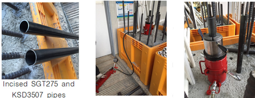
(b) Pullout capacity test of incised steel pipe
