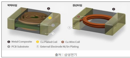
Fig. 2. Power Inductor Thin Film, Winding Type
