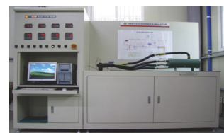
(a) Heat exchanger simulator
