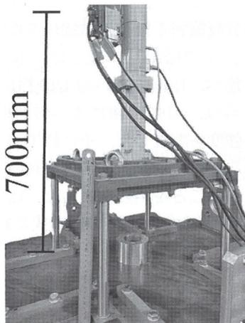
Fig. 4. Photo of consolidation testing machine. 압밀시험기기 사진.
