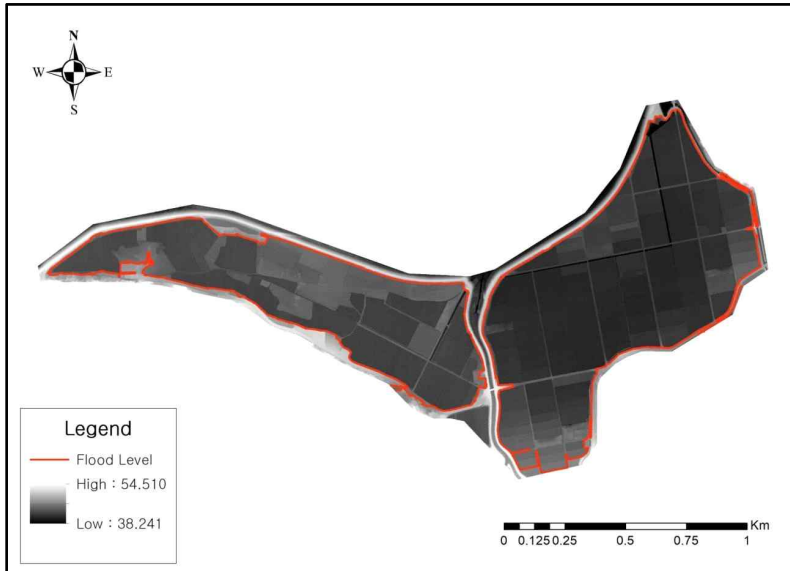
FIGURE 11. Creation of flood level line based on DEM
