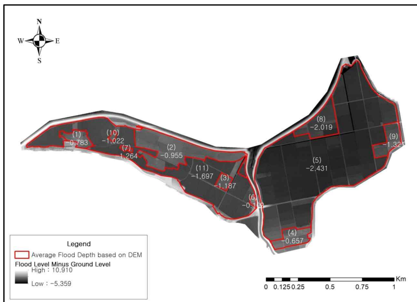
FIGURE 15. Average flood depth value obtained from DEM
