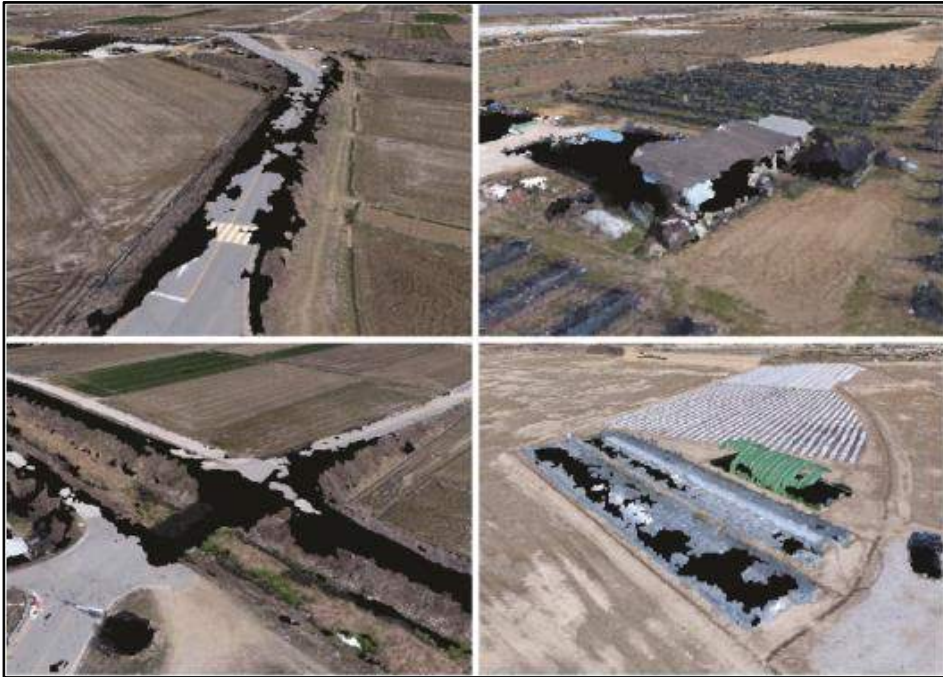
FIGURE 5. Class classification error in point cloud
