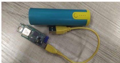
Fig. 8. MN and Power Supply
