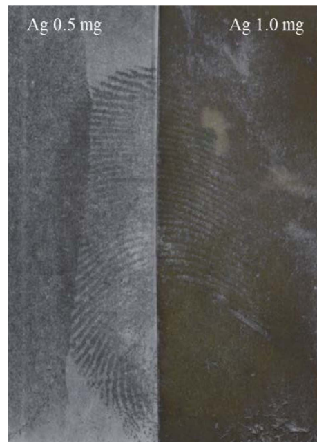
Fig. 1. Fingerprints left on wet paper developed by Ag-PD (left: 0.5 mg of silver deposited, right: 1.0 mg of silver deposited.).
