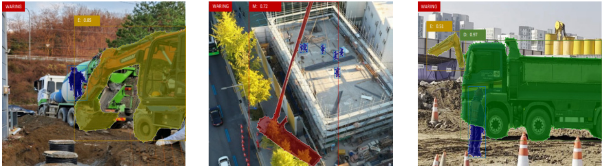
Fig. 6. Risk information notification screen when close to construction equipment and workers (continued)
