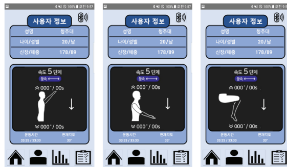
Fig. 4. Bluetooth application GUI according to the exercise area and mode when exercising.
