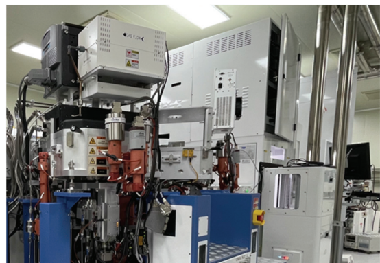
Fig. 2. A photograph of the PECVD chamber employed in this experiment (remote plasma case): Photo is taken from the authors at Myongji University).
