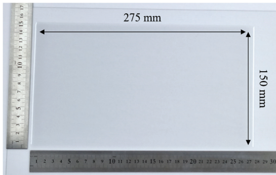
Fig. 4. Image of PDMS film coated using slot-die head with 100- \mu\text{m} -thick shim at the flow rate of 1 ml/min and the coating velocity of 1 mm/s.
