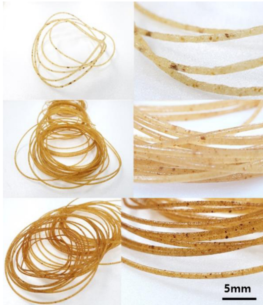
Fig. 1. Organic soybean hull - PLA composite filament according to the number of mixing repetitions (Top: 1 time, middle: 2 times, bottom: 3 times)
