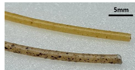
Fig. 4. Organic soybean hull - PLA composite filament according to the powder size (Top: fine powder, bottom: coarse powder)
