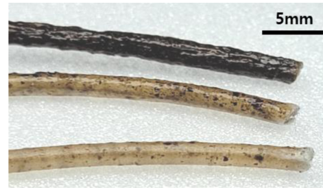
Fig. 3. Organic soybean hull - PLA composite filament according to the extrusion speed (Top: 10 rpm, middle: 15 rpm, bottom: 20 rpm)
