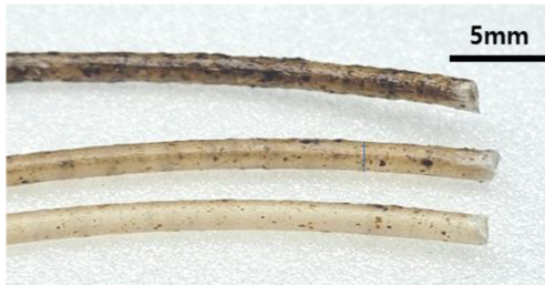
Fig. 2. Organic soybean hull - PLA composite filament according to the mixing ratios (Top: 10 wt%, middle: 3 wt%, bottom: 1 wt%)
