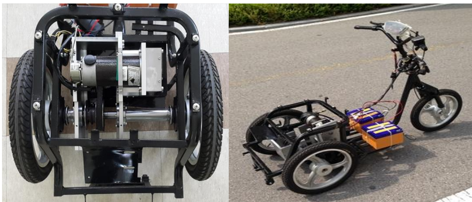
Figure 9. A small electric vehicle equipped modified CVT using spring
