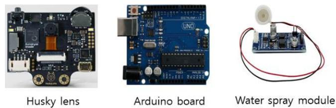
Figure 3. Main components of a scent dispensing system
