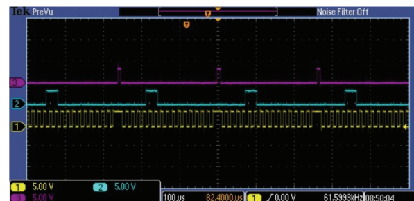
Fig. 1. Interface waveform for SPI communication.
