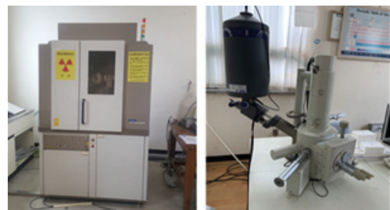
Fig. 3 (a) XRD(X-Ray Diffractometer) D/MAX 2200 (b) SEM, scanning electron microscopy (JEOL, JSM-5600) & EDX, energy-dispersive X-ray spectroscopy (JEOL, JSM - 6587)
