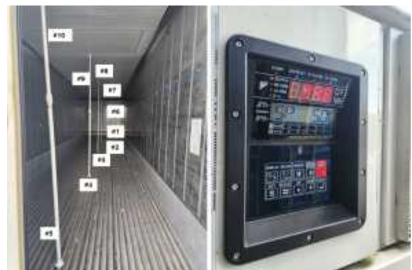
Fig. 2 Thermometer attachment location and freezer set temperature
