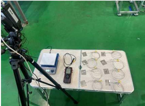
Fig. 4 Experiment setup for thermocouple test
