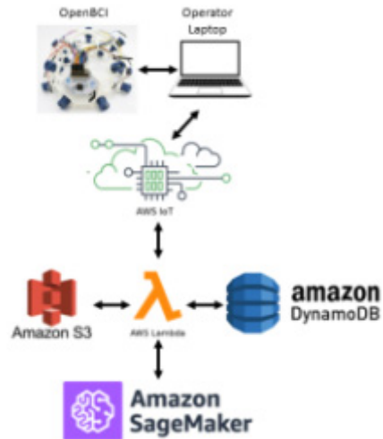
[Fig. 1] Brain-machine Interface System based on Cloud IoT Service [14]
