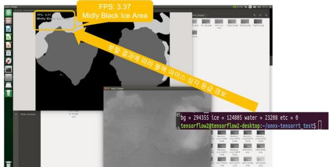
**Figure 11:** Black Ice Level Warning in Real-time on Jetson Nano
