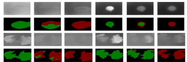
**Figure 9:** Example of original images and labeled or masked images of black ice generated on asphalt roads and cement roads for different cases
