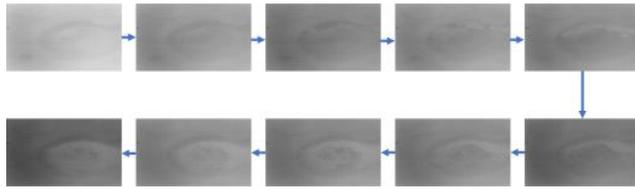
**Figure 7:** An example of the gradual formation of black ice on a wet road surface.
