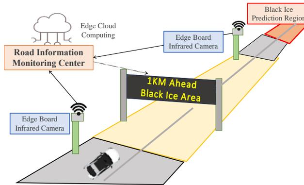
**Figure 1:** Illustration of a cloud-edge collaborative warning system of real-time road black ice
