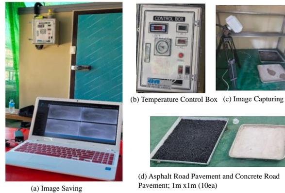
**Figure 5:** Experimental setup picture of Taking Images of Infrared Road Black Ice Experiment; (a) Image Saving, (b) Temperature Control Box, (c) Image Capturing, (d) Samples of Asphalt Road and Concrete Road Pavement.
