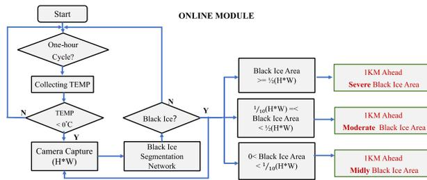
**Figure 4:** Workflow of Real-time Black Ice Region Warning Module
