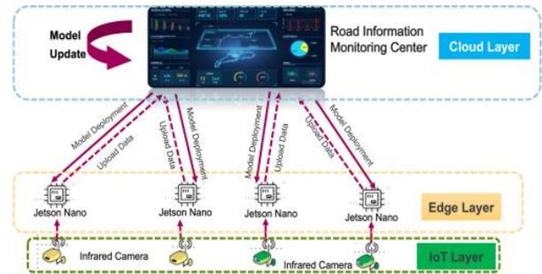
**Figure 2:** System Model of Cloud-edge Warning Collaborative System
