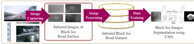
**Figure 3:** Illustration of black ice semantic segmentation training module (offline module)
