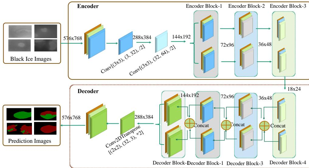
**Figure 6:** Encoder and Decoder Block Diagram of the Paralled Execution of Convolution with Multi-Scale Dilated Convolutional Feature Fusion (MsDC-FF) Module (Kang, S. 2023).
