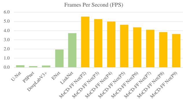
**Figure 10:** FPS comparisons of neural networks when using Jetson nano devices
