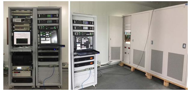
Fig. 3. eLoran transmitting and time synchronization systems.
