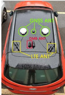
Fig. 9. Test road – mobile positioning system antenna setup.
