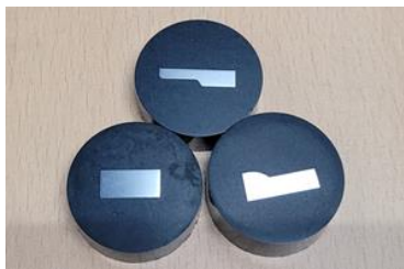
Fig. 7 Hardness test specimen of mandrel
