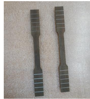
Fig. 9 Tensile test specimen of mandrel
