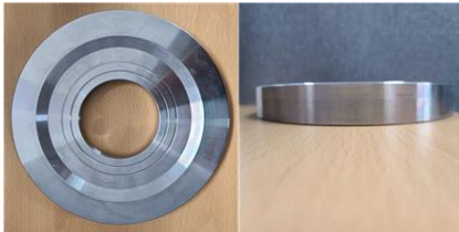
Fig. 1 Hot forged S20C preform
