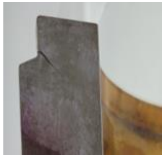
Fig. 13 Crack shape on the cross section of mandrel
