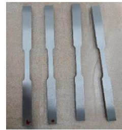
Fig. 3 Tensile test specimen of preform
