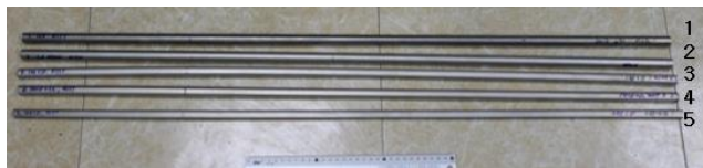
Fig. 3. Photos of as-received, annealed and cold-drawn \gamma -stainless steel
