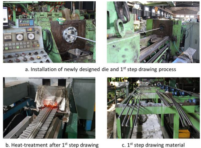
Fig. 21. Photos for representative flowchart showing 1 st step cold drawing followed by bright annealing
