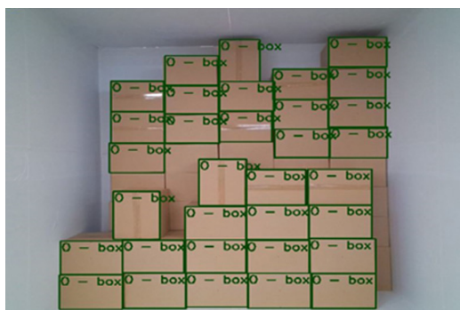
[Fig. 7] Result of box detection: the green squares denote the size and the location of detected boxes
