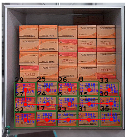
[Fig. 10] Result of unloading path planning in the first box layer: The red circle denotes the center location of a box, the red line shows optimal unloading path
