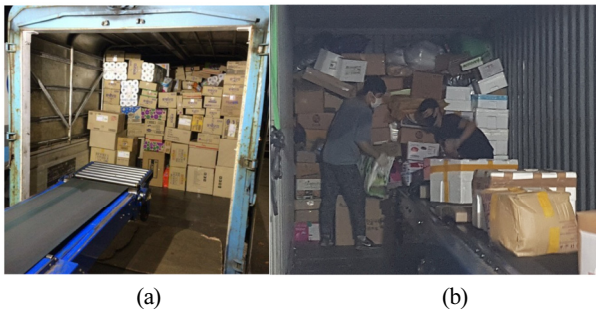
[Fig. 1] Real environment of trunk cargo box unloading: (a) A situation in which various types of boxes are stacked inside the cargo truck, (b) Scene with workers taking out boxes from trucks
